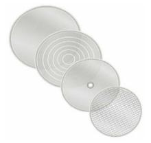
**Ultrasonic screens:** Designed for a growing niche of uniquely fine material applications (powders, minerals, etc.), sound wave frequencies move across the round screen wire to help overcome plugging to help increase throughput and efficiency. Midwestern supplies complete Ultrasonic systems for new equipment or your existing equipment for most makes and models of round separators.
