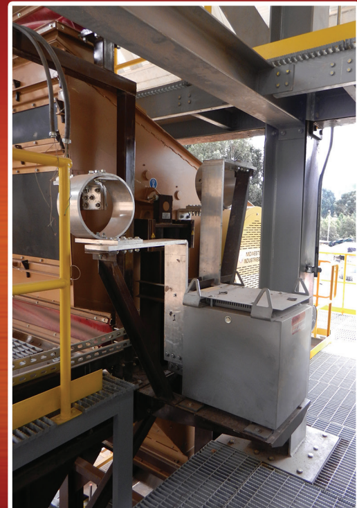
Screen heating installed on a Midwestern MEV®.
