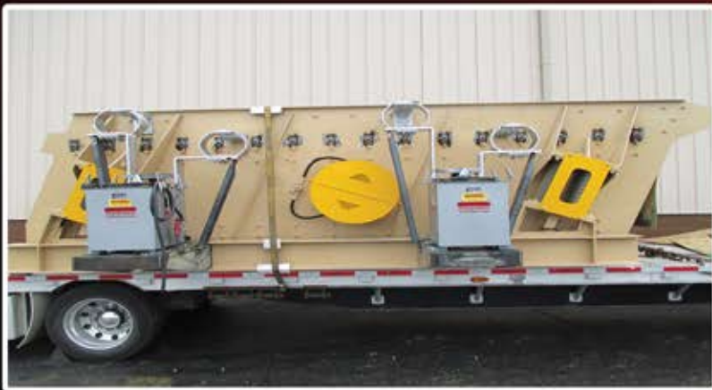
Two screen heating units installed on a non-Midwestern Industries screener.
