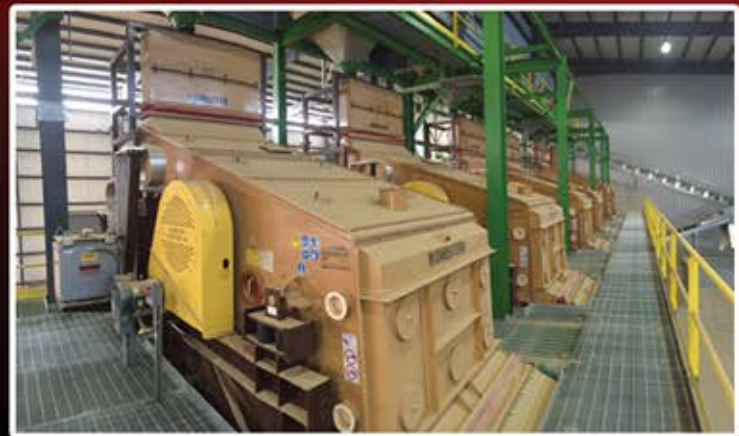
A brick plant utilizing screen heating on multiple MEV screeners.
