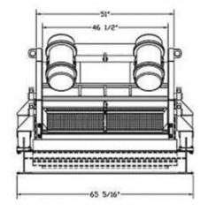
The Ultra-Vib is an ideal screener for dewatering applications. Optional spray bars can be added if needed.
